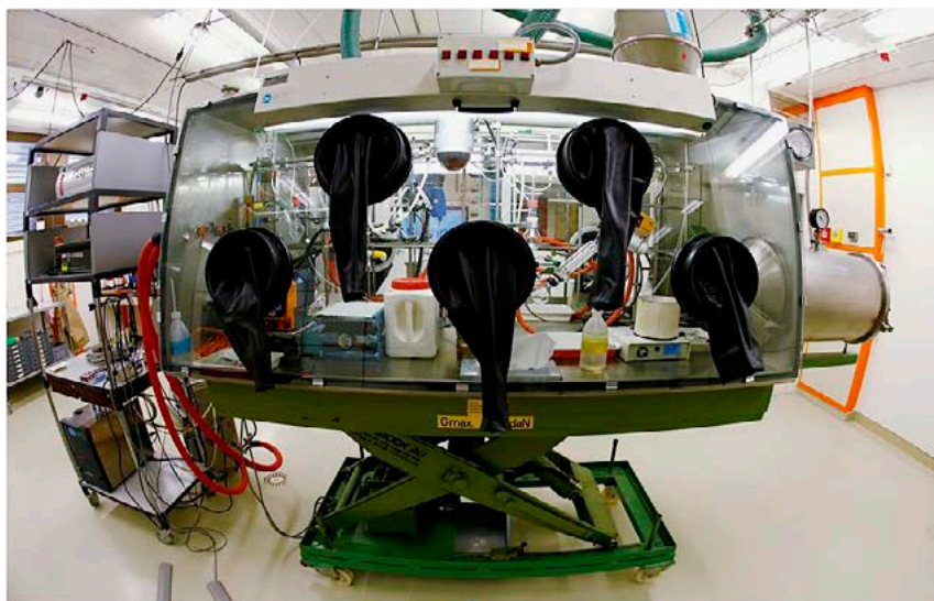
Glovebox for the synthesis of toxic chemicals
