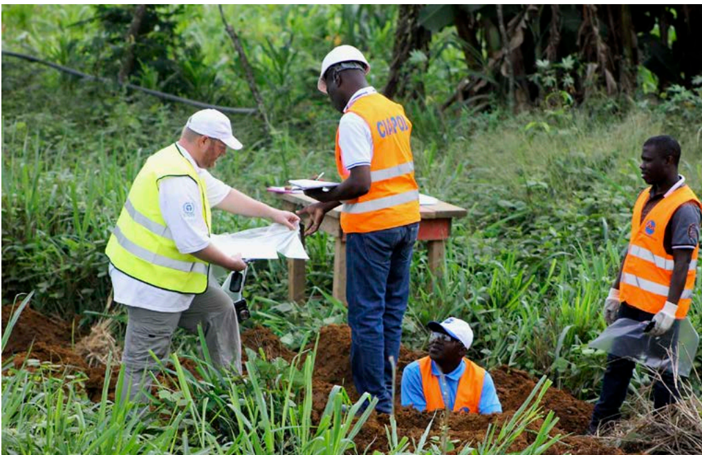
Soil sample collection at different depths at one of the cleaned-up sites
