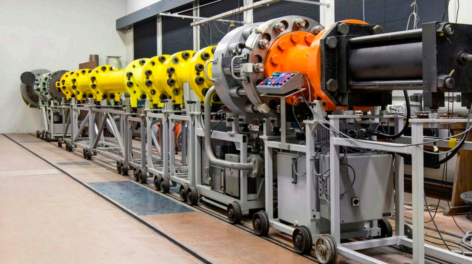
The research shock tube of the Collective Protection Branch at Spiez Laboratory
